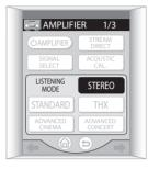
**STEREO** shows in the front panel display. Any active Advanced surround or Home THX mode is canceled. Dolby Digital and DTS multichannel sources are downmixed to stereo.
